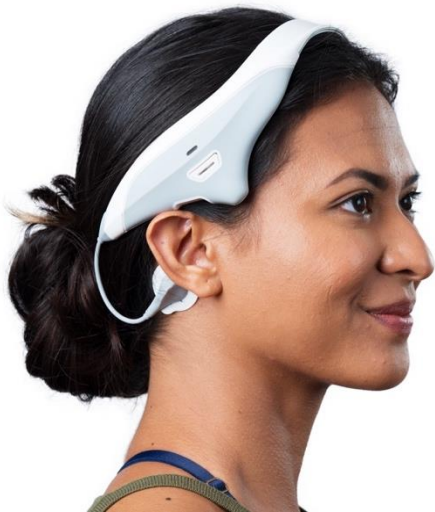
Photograph of the study device, showing the headset-style design and mastoid electrode placement.
